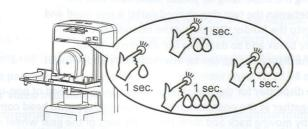
The dispensers recognize a hand approaching the trigger area by the double sensor and control electronics (only when the front cover is fully closed) and automatically trigger a dose.
